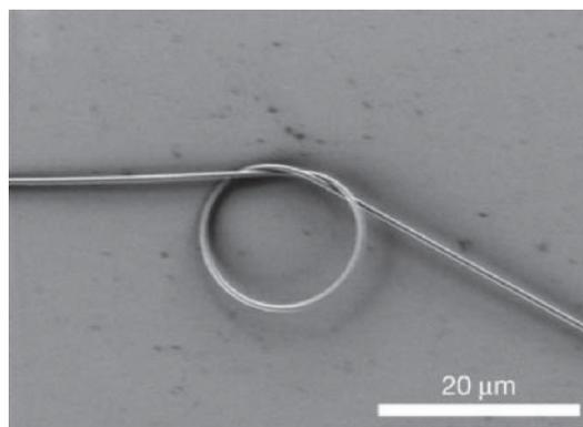
**Figure 1** Tong and co-workers demonstrate the flexibility and robustness of their silica nanowires by literally tying them in knots. This scanning electron micrograph shows a 15- $\mu\text{m}$  diameter micro-ring made with a 520-nm-diameter silica wire (from ref. 4).
