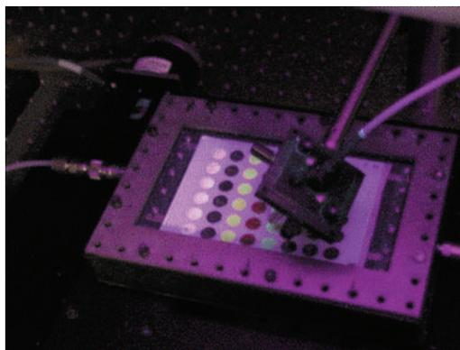
**Figure 1** Sensor array testing. The sensing ability of organic thin-film formulations is evaluated with an optical scanning probe that measures their reflectance or fluorescence and relates these properties to the film performance. The films in this array are formulated to be responsive to environmental parameters such as the composition of chemical vapours that flow over them.
